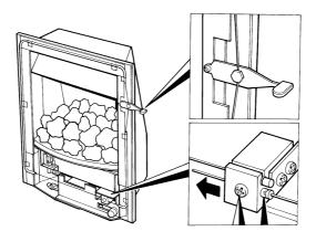
g) Unscrew the burner assembly fixing screws at either side of the firebox, and the two fixing screws at the base of the fire (See fig. 7 below). Carefully pull the base of the burner forwards. The burner can now be removed from the appliance.
