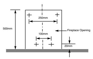
Fit the wallplugs provided and screw the fixing eyes securely into the rear of the fire opening.
